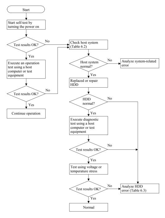
Figure 6.1 Test flowchart
